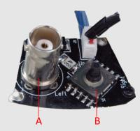
A. The second video out on the board allows user to use a test monitor to adjust the camera without connecting the camera to the security system.
